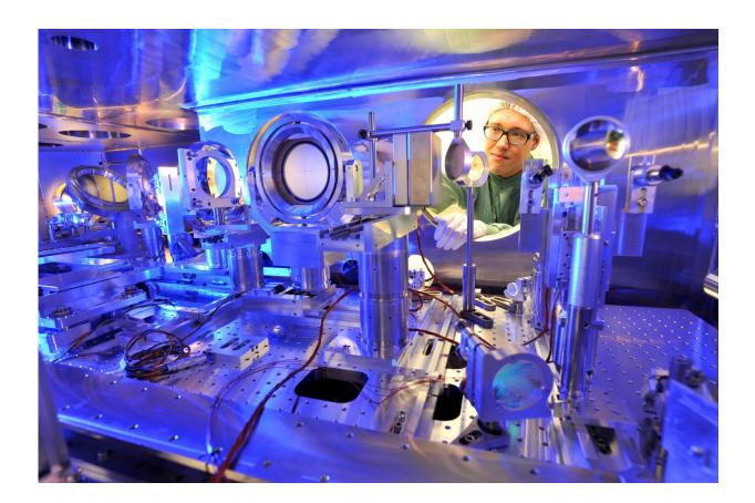
In a target chamber, the light pulse of the high-performance laser DRACO hits a gas-jet. The aim is to accelerate electrons to almost the speed of light on a distance shorter than a pencil's width. Credit: HZDR / F. Bierstedt
