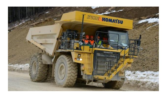
Until last year, the Komatsu dumper truck chugged around the cement works quarry powered by its Diesel engine. In a few months, it will be expected to do the same job running purely on electricity. Credit: Andreas Sutter, Lithium Storage GmbH
