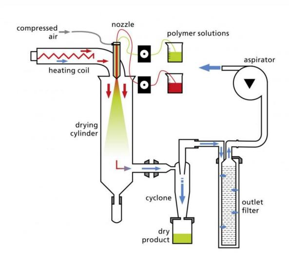
Schematic diagram of the spray-drying process. Credit: Fraunhofer IGB
