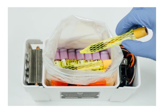
Temperature-controlled specimen transport container designed by Johns Hopkins researchers is packed with blood sample test tubes. Credit: Johns Hopkins Medicine
