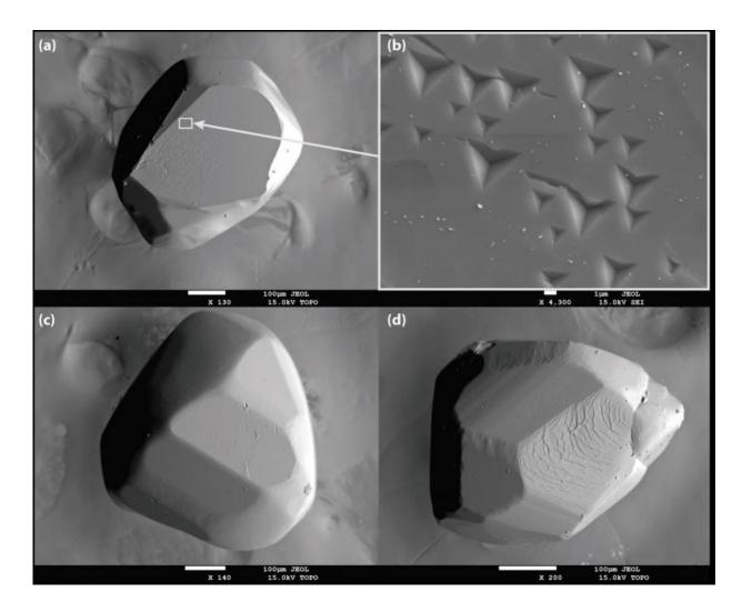
Electron microprobe images of inclusions. (a, c) show diamond imposed cubooctahedral morphology. The surface of V471 (b) has trigonal features that establish that the inclusion and host diamond formed simultaneously. The top surface of V405 (d) records stepped features and the side faces show well developed growth lines consistent with simultaneous growth with the host diamond. Credit: Koornneef et al
