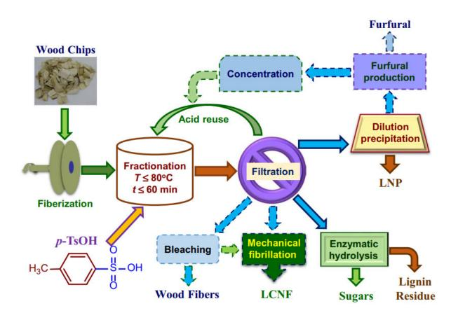
Schematic flow diagram shows wood fractionation using p-TsOH for the production of fibers, lignocellulosic nanomaterials, sugars, and LNPs. Processes with dashed lines were not carried out in this study. Credit: *Science Advances* (2017). DOI: 10.1126/sciadv.1701735
