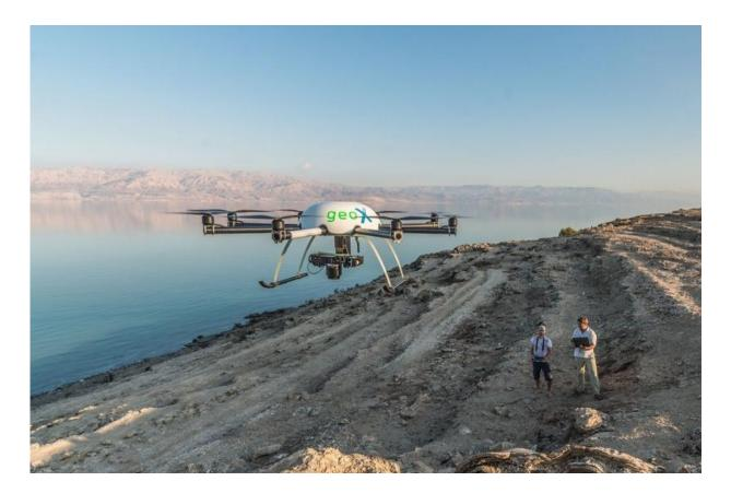
Octocopters produce aerial and thermal photographs of excellent threedimensional resolution. Scientists use them for digital terrain models to identify underground feeders of groundwater. Credit: André Kuenzelmann, UFZ
