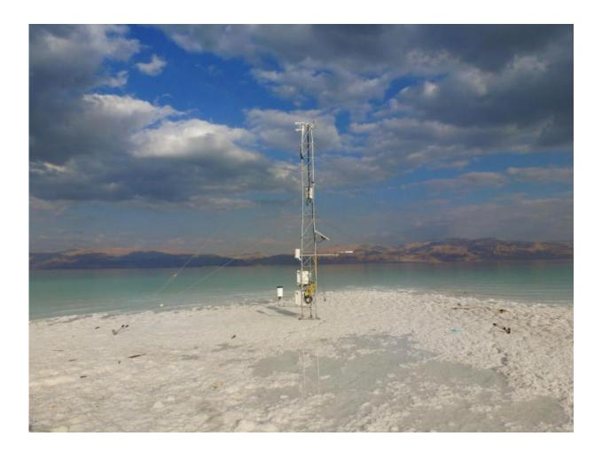
The world's lowest meteorological station located at 429 m below sea level continuously measures evaporation of water of the Dead Sea. Credit: U. Corsmeier, KIT
