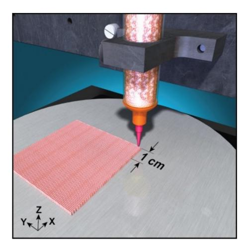
The researchers printed their silicone-based samples using a direct-ink writing process. The composite ink material was extruded at room temperature from the printer's nozzle to form woodpile-like structures with controlled porosity and architecture. Credit: Lawrence Livermore National Laboratory
