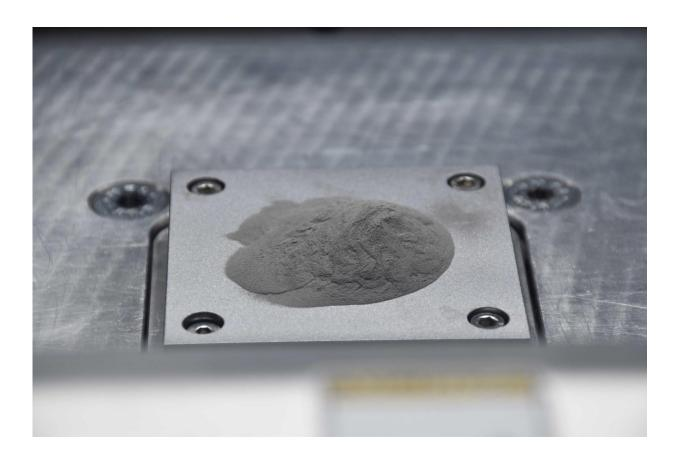
The nanoparticle-functionalized powder is fed into a 3-D printer, which layers the powder and laser-fuses each layer to construct a three-dimensional object. Credit: B. Ferguson - HRL Laboratories
