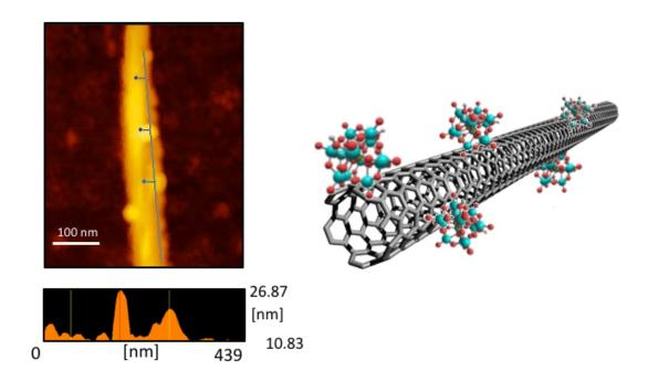
Researchers have demonstrated that functionalizing SWNTs with phosphomolybdic acid generates a large and tunable type of electrical noise that
