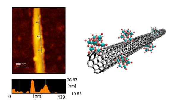
Researchers have demonstrated that functionalizing SWNTs with phosphomolybdic acid generates a large and tunable type of electrical noise that
