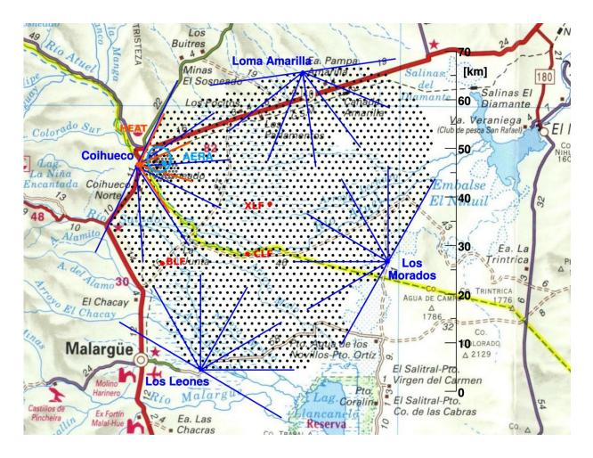
This map depicts the placement of the surface detectors in the array. Credit: Pierre Auger Observatory
