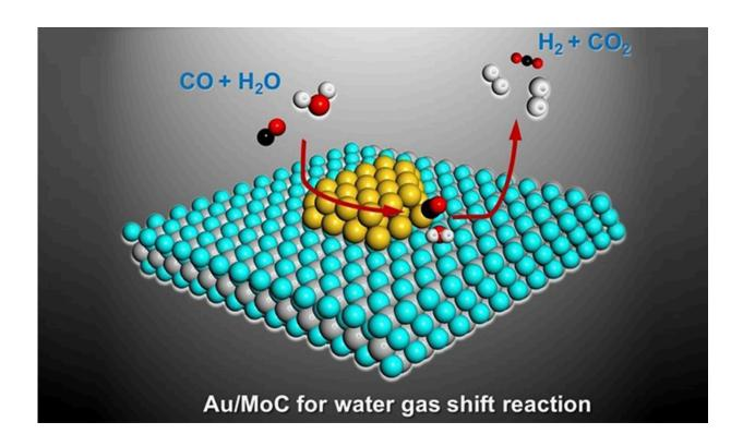
An international research group, including materials scientists from Lehigh, has developed a gold-based catalyst that converts carbon monoxide and water into a stream of pure hydrogen and carbon dioxide. Credit: Ding Ma/Peking University and Chemistry World
