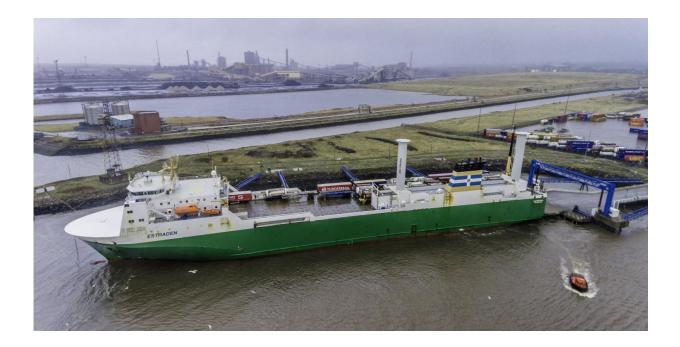
Spinning cylindrical sails can be used on large ships to reduce greenhouse gas emissions and propel them forward. Credit: Norsepower
