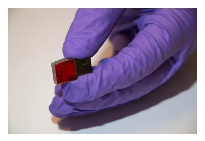
MIT postdoc Itai Stein holds samples of cured phenolic resin and glassy carbon. Credit: Denis Paiste/Materials Processing Center
