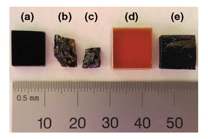
Samples of carbon nanotubes and polymeric phenol-formaldehyde materials hardened through baking at high temperature in the absence of oxygen: (a) a carbon nanotube forest; (b) a carbon nanotube/polymer nanocomposite; (c) a charcoal-like carbon nanotube/glassy carbon nanocomposite after baking at high temperature; (d) pure polymer (phenol-formaldehyde); (e) a charcoal-like glassy carbon block from baking a polymer at high temperature. Credit: Ashley Kaiser and Itai Stein
