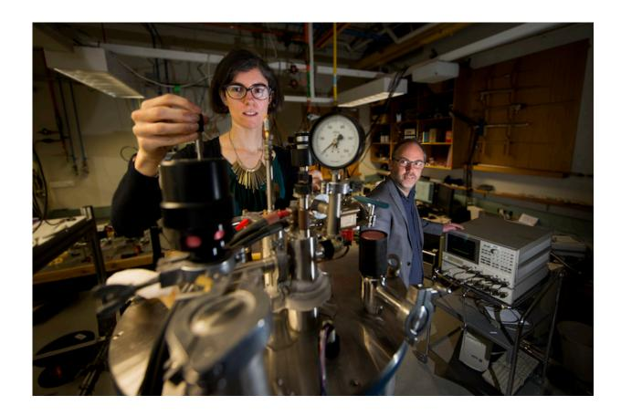
Dr Rose Ahlefeldt and A. Prof Matthew Sellars operating a superconducting magnet cryostat, used in the experiment to generate a high magnetic field and extremely low temperatures Credit: ANU/cqc2t.org
