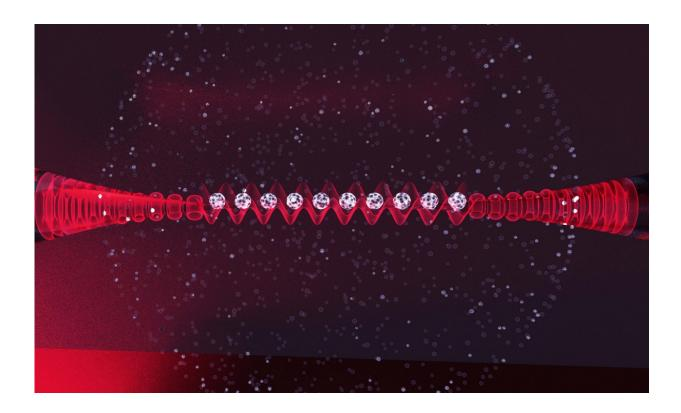
Cartoon graphic of a nanoscale optical fiber immersed in a chilled gas of atoms. Atoms from the gas are caught by the wiggles of light that surround the narrowest part of the fiber. Light waves propagating down the fiber both capture and probe the atoms, allowing scientists to study interesting light-matter physics. Credit: E. Edwards/JQI
