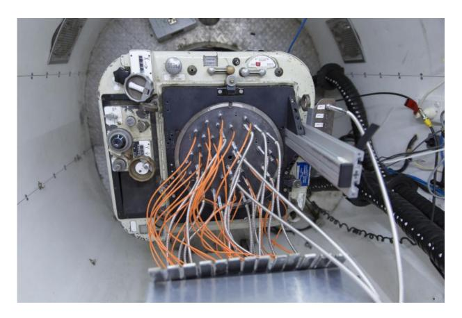
The SAMI instrument at the 3.9m Anglo-Australian Telescope. Each silver cable holds a 'hexabundle' of special optical fibres that can look at several different points across the face of a single galaxy. SAMI can study 13 galaxies at a time. The orange cables also hold optical fibres: these are used for calibration purposes. Credit: Ángel R. López-Sánchez.
