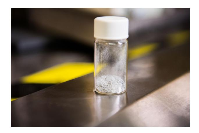
Army scientists and engineers found that a nano-galvanic aluminum-based powder they developed produces hydrogen when added to water or any liquid containing water. Credit: David McNally, ARL Public Affairs
