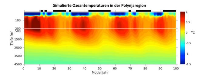
Simulated temperature development in the area of the polynya. Clearly marked are the cold isolating surface layer (blue) and the warm water (red) below that releases head to the atmosphere on decadal cycles. Years with polynyas are marked by a black bar at the upper boundary. Credit: Helmholtz Association of German Research Centres
