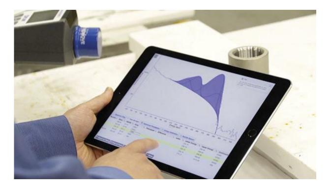
InterSpec, available for both mobile and traditional computing devices, can quickly analyze gamma radiation data. The tool was developed by Sandia National Laboratories. Credit: Sandia National Laboratories
