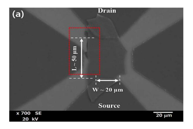
Scanning electron microscopy image of the near-infrared photodetector based on few-layered MoSe<sub>2</sub>. Credit: University of Electro Communications
