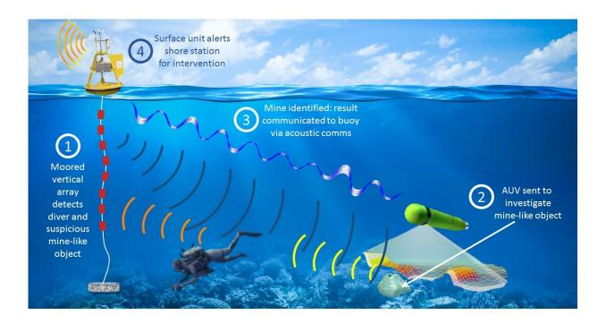
ThreatDetect's system concept: 1) Moored vertical array detects diver and suspicious mine-like object; 2) AUV sent to investigate mine-like object; 3) Mine identified: result communicated to buoy via acoustic comms; 4) Surface unit alerts shore station for intervention. Credit: ThreatDetect Project, IMDEA Networks Institute
