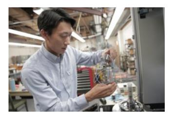
At UW-Madison, Hiroki Sone prepares a rock sample for deformation measurements under stress conditions in a triaxial rock mechanics apparatus. Credit: Stephanie Precourt.
