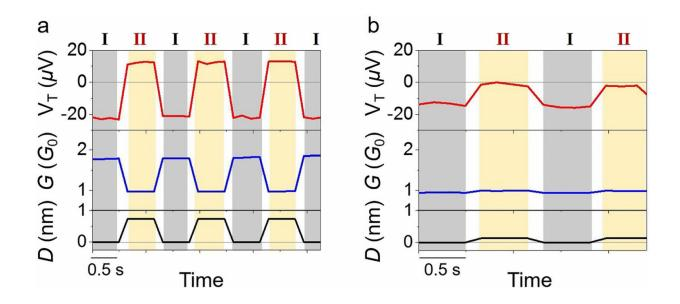
Control of thermoelectric voltage (VT) and conductance (G) with the periodic variation of elongation of the contact (D). The elongations in (a) and (b) were 0.73 nm and 0.10 nm with temperature differences of 10 K and 4.4 K, respectively. Credit: *Scientific Reports*
