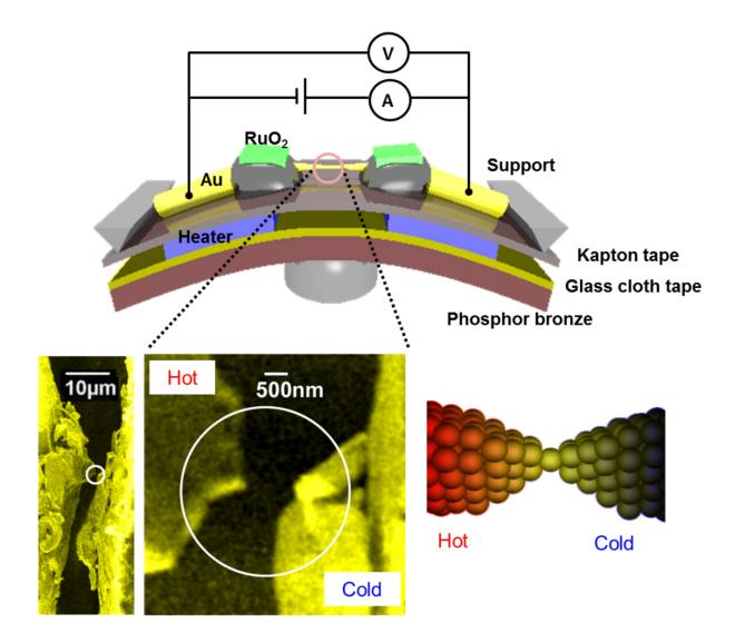
Schematic view of the experimental setup. The inset shows microscopic images of the contact after it is broken by elongation. Credit: *Scientific Reports*
