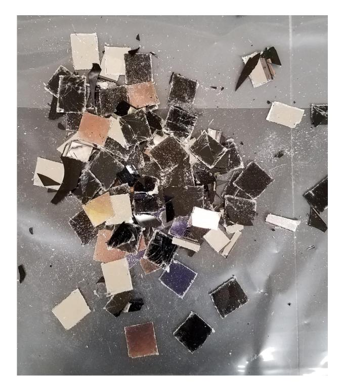
Quantum-dot-containing tablets and TVs were carved into small pieces and then placed into a simulated landfill to see whether the dots would leach into the environment. Credit: Yuqiang Bi
