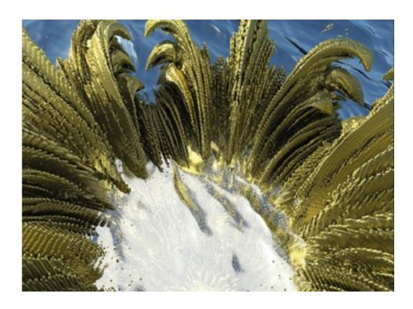
A nanostructured metamaterial with a sunflower-like arrangement can be immersed in water to generate hydrogen gas with superb efficiency. Credit: WILEY-VCH Verlag GmbH & Co.
