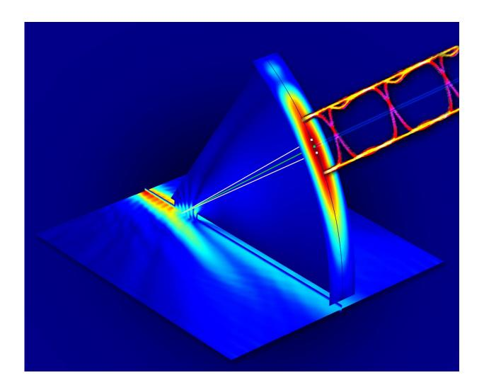
Multiplexing, the ability to send multiple signals through a single channel, is a fundamental feature of any voice or data communication system. An international research team has demonstrated for the first time a method for multiplexing data carried on terahertz waves, high-frequency radiation that may enable the next generation of ultra-high bandwidth wireless networks. The image
