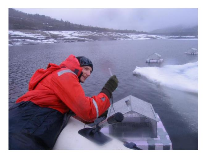
Greenhouse gas measurements in a Norwegian reservoir in early spring. SINTEF scientist Bjørn Henrik Hansen is using syringes to sample gas from floating chambers. Credit: Norway
