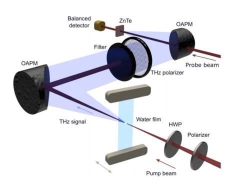
Experimental setup for generating THz waves by focusing a laser beam onto a free-flowing water film. Credit: Jin et al. ©2017 American Institute of Physics
