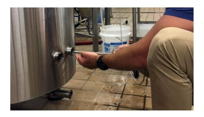
Ph.D. student Lucas Vann inserts a sensor into a fermenter. The sensor offers brewers real-time data on the fermentation process. Credit: North Carolina State University
