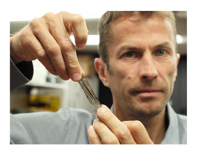
In this photo, IBM scientist Dr. Mark Lantz, holds a one square inch piece of Sony Storage Media Solutions sputtered tape, which can hold 201 Gigabytes, a new world record. Credit: IBM Research
