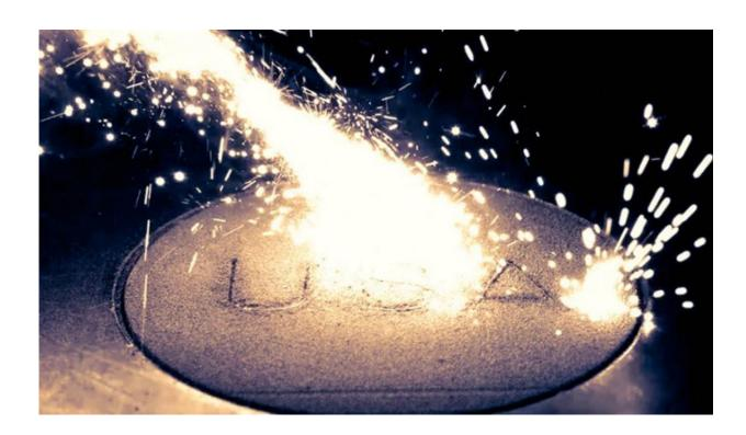
High-speed images of a common laser-based metal 3D printing process, coupled with newly updated computer models, have revealed the mechanisms behind material redistribution, a phenomenon that leads to defects in printed metal parts. Credit: Lawrence Livermore National Laboratory
