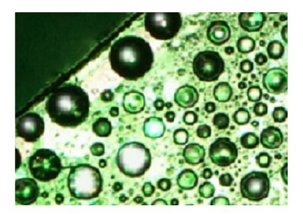
Water droplets form on a surface: the edge matters more than the surface wettability. Credit: KAUST
