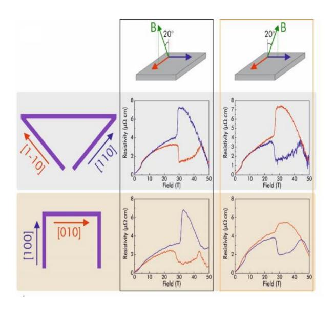
Carefully aligned microstructured devices of CeRhIn5 enabled high field transport measurements that reveal an in-plane symmetry breaking for magnetic fields of approximately 30 Tesla along the tetragonal c-axis. The anomaly size and direction is determined by a small in-plane component of the magnetic field.
