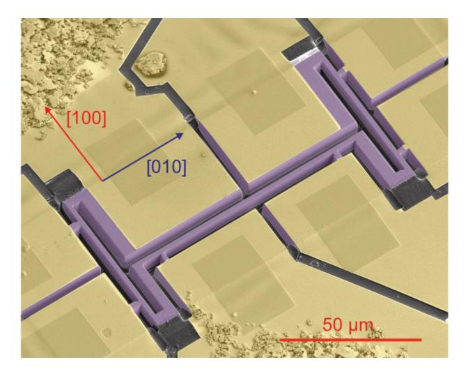
Crystalline samples of CeRhIn5 from Los Alamos were cut into microscopic, crystalline conducting paths with a focused ion beam at MPI-CPfS. Credit: MPI CPfS
