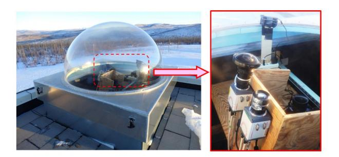
High-speed cameras installed at the Neal Davis Science Operations Center at the Poker Flat Research Range of the University of Alaska. Credit: NIPR
