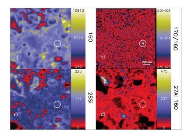
Detected for the first time: Image (b) shows a hotspot comprising an approximately 130-nanometre silicate stardust grain. Many stardust grains of this size only become visible when using the reduced ion beam. The image shows the isotope abundances of oxygen 16 (a) and silicon 28 (c) as well as the ratios of oxygen 17 to oxygen 16 (b) and of aluminum 27 to oxygen 16 (d) for a 5 by 5 micrometre-sized region in the QUE 99177 meteorite, which was found in
