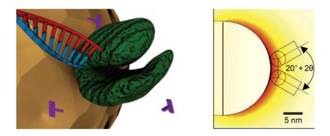
Lending a hand: The sensor is able to detect when a DNA polymerase molecule binds to the gold nanorod of a plasmonic nanosensor and synthesises a DNA strand. During this process the enzyme opens and closes like a hand, changing
