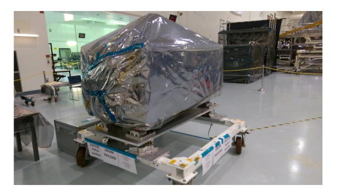
The ISS-CREAM payload was delivered to NASA's Kennedy Space Center in August 2015. The experiment is shown wrapped in plastic layers used to protect its sensitive electronics during shipment. Credit: University of Maryland Cosmic Ray Physics Laboratory
