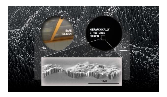
A Lawrence Livermore National Laboratory team lead by Anna Hiszpanski has devised guidelines for an alternative to anti-reflective coatings on optical devices such as solar cells, glasses and cameras, by engineering their surfaces with layers of hierarchical micro- and nanometer length structures. Credit: Lawrence Livermore National Laboratory
