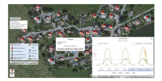
With one click, the researchers can visualize what is happing to voltage if a photovoltaic system is built in the district. Credit: Adaptricity
