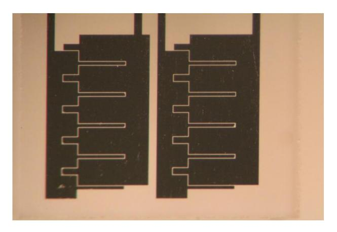
A close-up view of the lead sensor, featuring two pairs of electrodes. It could enable cities and homeowners to pinpoint pipes that taint water with lead. Credit: Wen-Chi Lin, Burns Lab, University of Michigan
