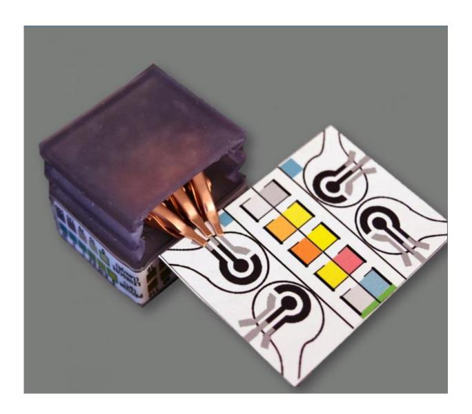
New paper-based diagnostic device detects biomarkers and identifies diseases by performing electrochemical analyses, and the assays change color to indicate specific test results. The device can plug into a handheld potentiostat, at left, to
