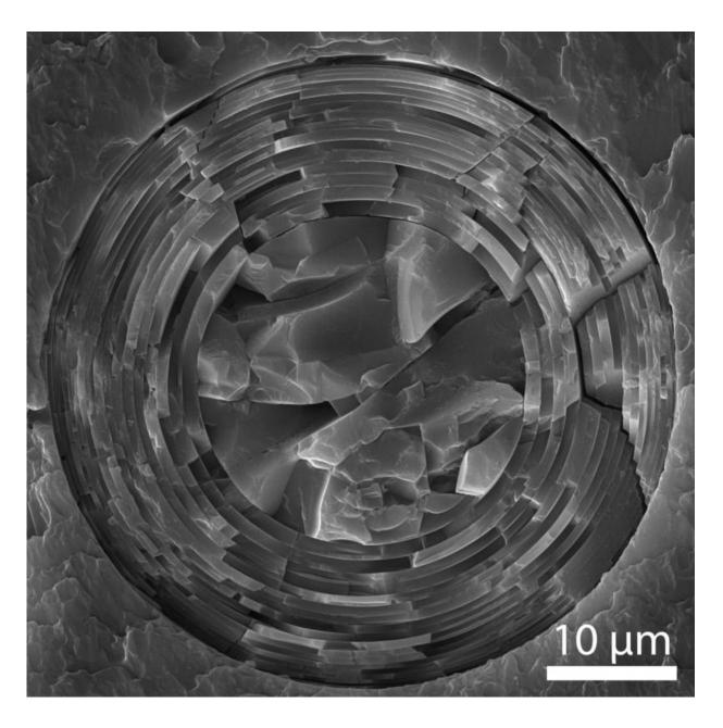
A cross-section of an Euplectella aspergillum spicule showing the arrangement of microscopic concentric layers of glass inside it. Credit: James C. Weaver/PNAS, CC BY-ND
