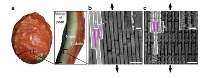
A cross-section from a red abalone (Haliotis rufescens) shell shows its brick wall mechanical design. Credit: Espinosa et al., Nature Communications 2, 173 (2011), CC BY
