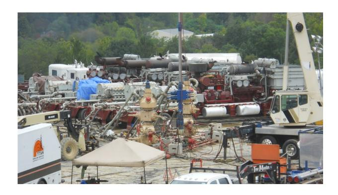
Hydraulic fracturing operations (here, in western Pennsylvania) inject mixtures of pressurized water, chemicals and sand mixture underground to fracture rock and release trapped oil and natural gas. EPA has warned that poorly managed fracking operations could contaminate drinking water. Credit: Doug Duncan, USGS
