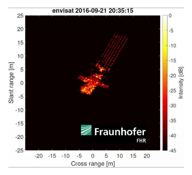
A correctly scaled radar reconstruction of the ENVISAT satellite. Credit: Fraunhofer FHR
