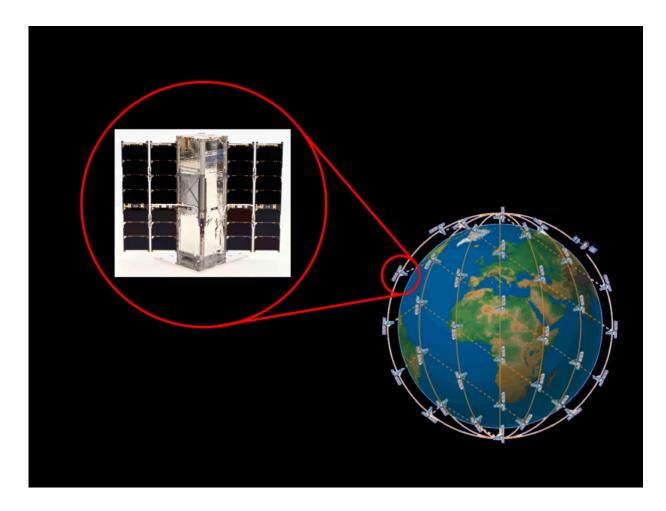
Radiometer Assessment using Vertically Aligned Nanotubes, or RAVAN, is a 3-unit CubeSat that successfully demonstrated new technologies for measuring the amount of reflected solar and thermal energy that is emitted into space. These observations have the potential to improve spaceborne measurements of Earth's energy imbalance. Credit: Johns Hopkins University Applied Physics Laboratory
