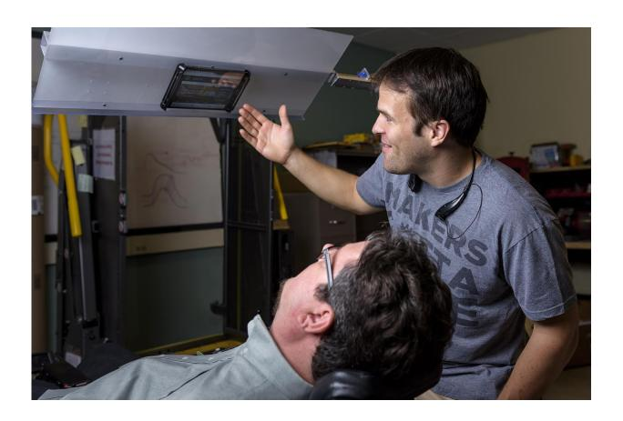
Brad Duerstock and Jeffrey Ackerman developed RoboTable with funds from the U.S. Department of Veteran Affairs' Specially Adapted Housing (SAH) Assistive Technology Grant. This robotic arm acts as an over-the-bed platform capable of mobilizing users' mobile devices or laptop computer while they are restricted to bed. Duerstock (left) and Ackerman (right) demonstrate RoboTable's ability to adjust for a reclined user's needs. Credit: Purdue Research
