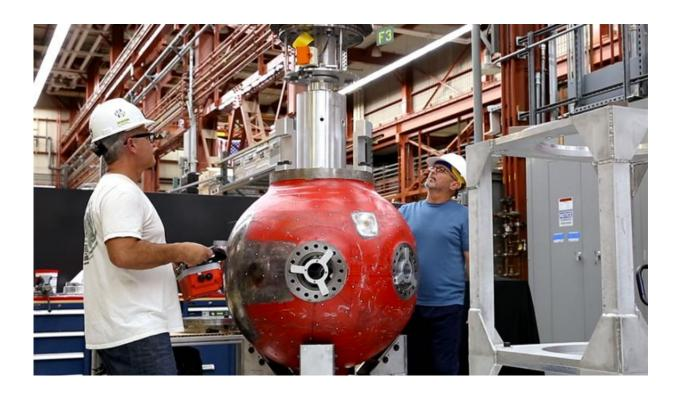
Senior mechanical Technician Rich Moore (left) and Mechanical Designer Kevin Morris lower an alignment mechanism into a vessel that confined an experiment with conventional explosives and mock parts that took place Monday. It was the fourth of five preparatory experiments designed to confirm safety features leading up to a subcritical (unable to sustain the nuclear fission chain reaction) experiment with plutonium. Credit: Lawrence Livermore National Laboratory
