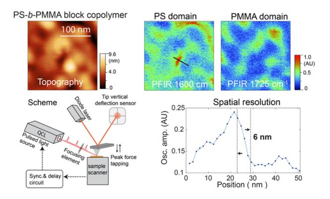
The lower portion of this image by Xiaoji Xu's group shows the operational scheme of peak force infrared (PFIR) microscopy. The upper portion shows the topography of nanoscale PS-b-PMMA polymer islands on a gold substrate. Credit: Xiaoji Xu
