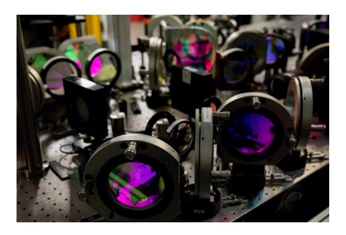
Highly reflective mirrors and telescope lenses in the Matter in Extreme Conditions (MEC) optical laser system are carefully positioned to propagate the instrument's high-quality laser beams. The laser beams create extreme pressure and temperature conditions in materials that are instantaneously probed using hard X-rays from SLAC's Linac Coherent Light Source (LCLS). Credit: Dawn Harmer/SLAC National Accelerator Laboratory
