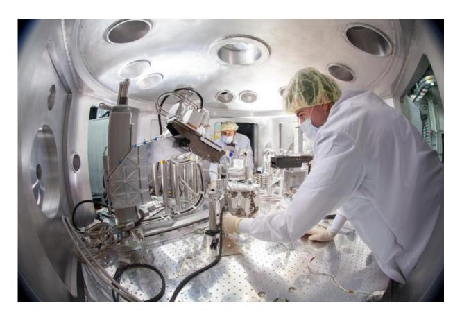
Inside the MEC vacuum target chamber where researchers create transient states of matter using high-power optical lasers, which are then examined with SLAC's Linac Coherent Light Source (LCLS) X-rays. Credit: Matt Beardsley/SLAC National Accelerator Laboratory
